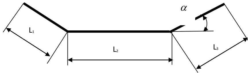
Fig.3. The mechanism of a direction of a mesh plane. \alpha – angle of slope, L_1, L_3 – the inclined parties of the directing mechanism, L_2 – the horizontal party of the directing mechanism.
